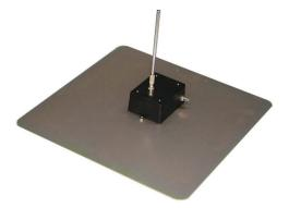
Frequency Range: 9 kHz - 40 MHz Impedance: Calibrated for use into 50 Ω Pattern Type: omni-directional Connector: BNC-Type, female Mounting Base: 1/4 - 20 Thread, female
