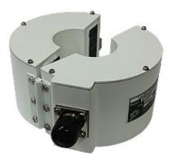
$\begin{array}{c} \mbox{Frequency Range: 1 MHz} - 500 \mbox{ MHz} \\ \mbox{Insertion Loss: 4 to 16 dB} \\ \mbox{Transfer Impedance: 16 to 31 dB} \\ \mbox{Rated Watts: 200 watts CW} \\ \mbox{Connector: N-Type, female} \end{array}$
