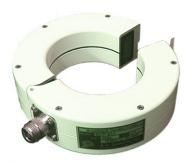
Frequency Range: 100 Hz - 100 MHz Transfer Impedance  $(dB\Omega)$ -90 to -43 Max Primary Current CW 60 Amps Max Primary Current 300 Amps (at 400 Hz) Max Primary Current Peak 5,000 Amps Connector: N-Type, Female
