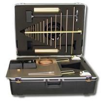
Frequency Range:20 Hz - 2 GHz Impedance:50 Ω Physical Dimensions Antenna Kit:28" x 23" x 10" (35 lbs.) Tripod Carrying case:46" x 8" Dia. (19 lbs.)
