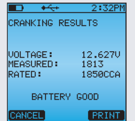
GENERATOR START Test the state of health of generator starting batteries.
